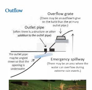
Common outlet variations designed to improve performance, reduce cost, and/or increase efficiency
