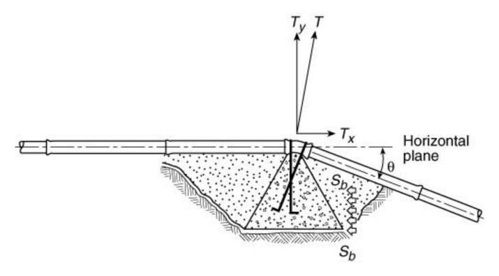
T = thrust force resulting from change of direction of flow
