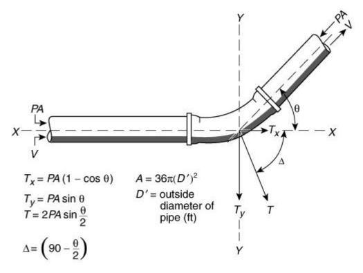
T = thrust force resulting from change in direction of flow (lbf)
