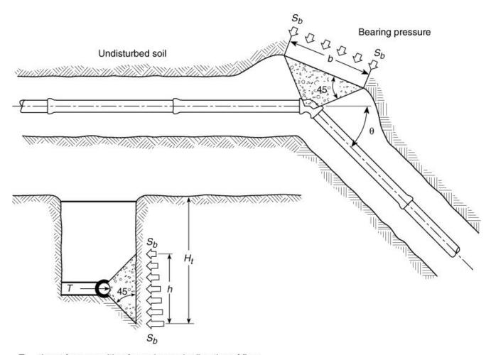
T = thrust force resulting from change in direction of flow
