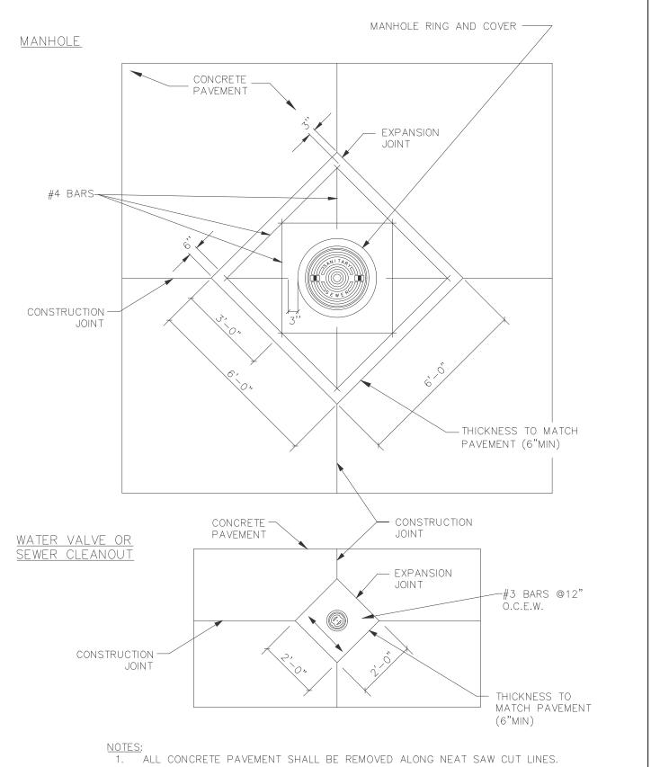
2. MANHOLE BOXOUT REQUIRED FOR ALL MANHOLES (STORM AND SANITARY), VALVES, AND CLEANOUTS LOCATED IN THE STREET.
